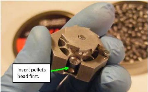
9. Move the star wheel counter-clockwise to continue filling each chamber.
