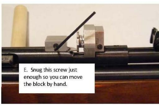
5. Fine tune the position of the indexing lever block as follows:
