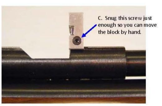
3. Place the magazine into the magazine block. Adjust the position of the magazine block so the magazine fits as closely to the front wall of the loading port as possible, then tighten the screw.
