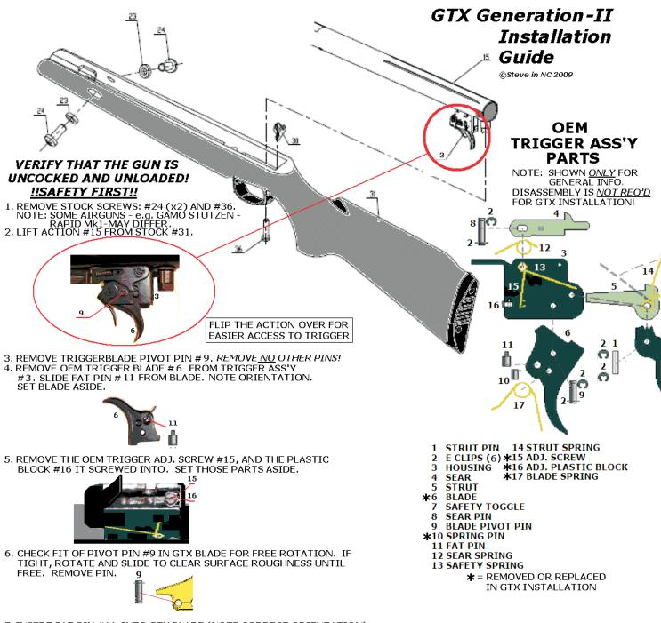
7. INSERT FAT PIN #11 INTO GTX BLADE (NOTE CORRECT ORIENTATION). FROM STEP #4.
